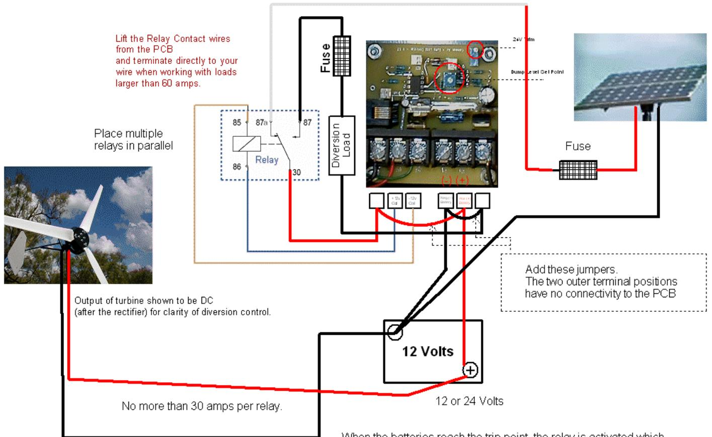
When the batteries reach the trip point, the relay is activated which opens the N/C circuit from the solar panels into the batteries.
