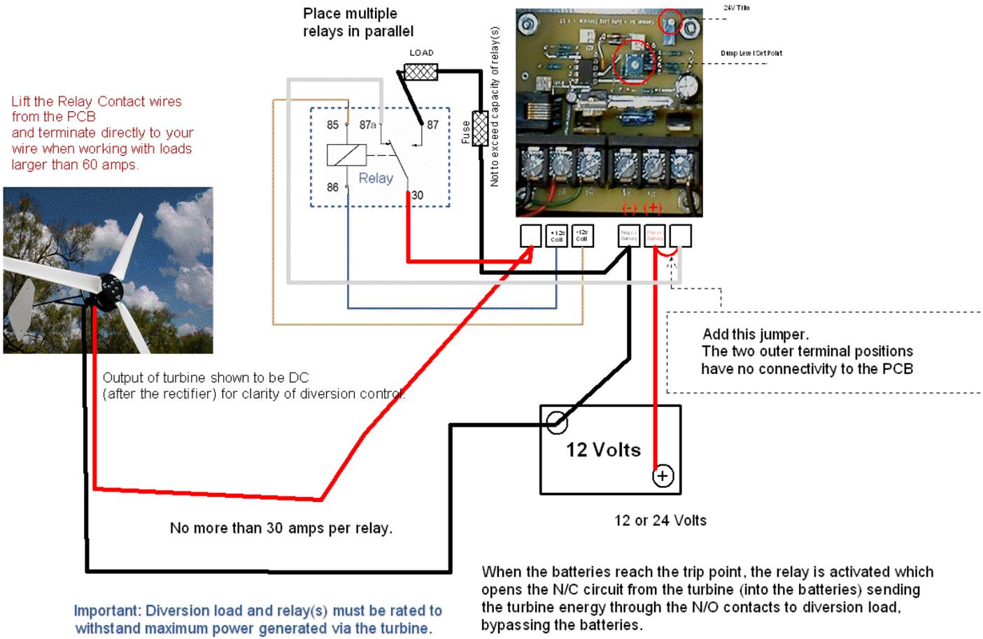
This wiring method is similar to the standard diversion control wiring, except that when the trip point is reached, power from the charge source (wind/solar etc) is no longer allowed to reach the batteries, but instead is sent directly to the diversion load. Use this method if you want your turbine to see a larger load when the batteries are full, possibly causing a slow down in your turbine RPM. Please see the notes about diversion philosophy in the earlier portions of this manual.
