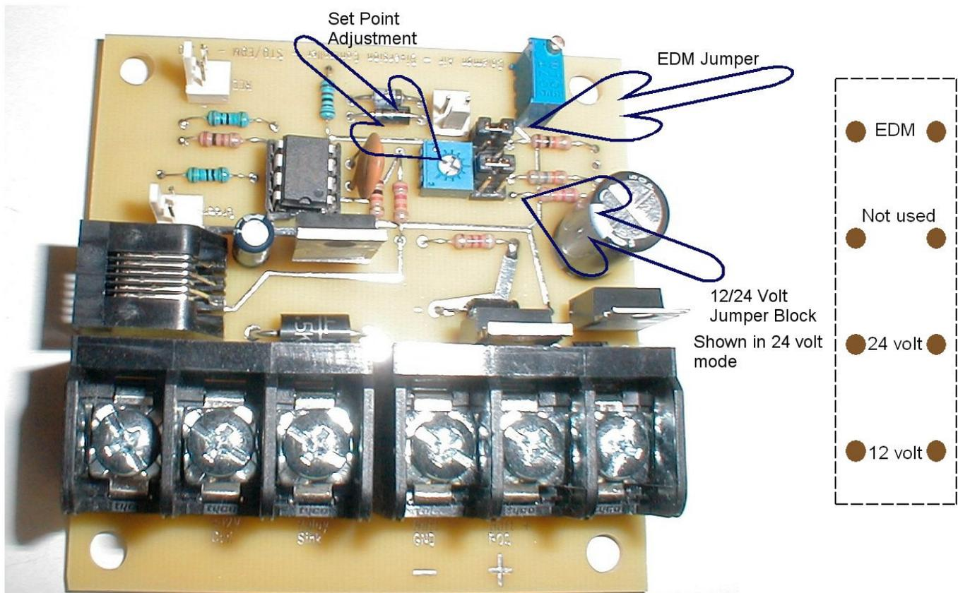
For a 24 volt battery bank, set the jumper in the 2<sup>nd</sup> position. (As shown in the image above.)
