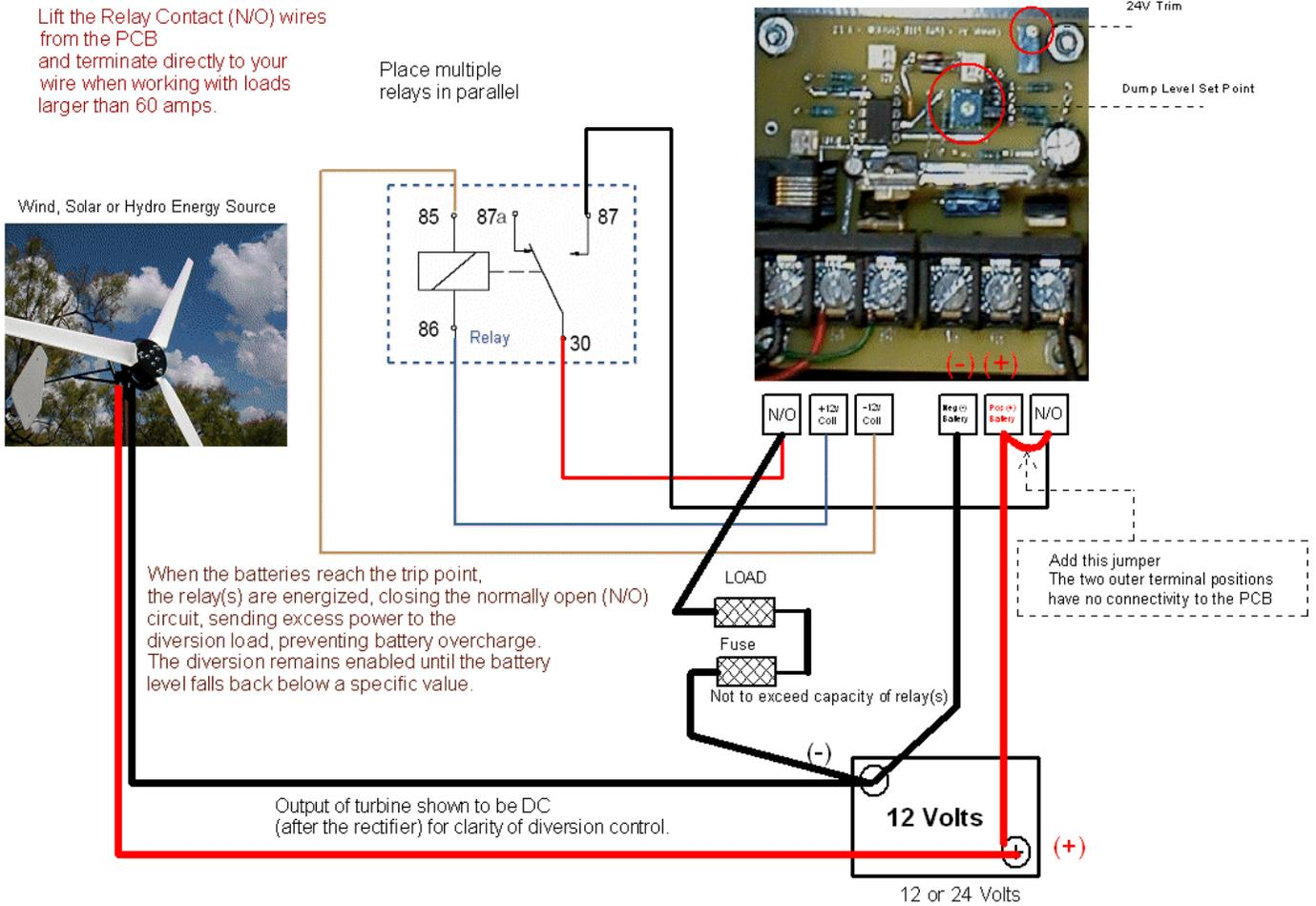
**This is the most used hookup method, particularly for wind and hydro units. This wiring method is also suitable for solar.**
