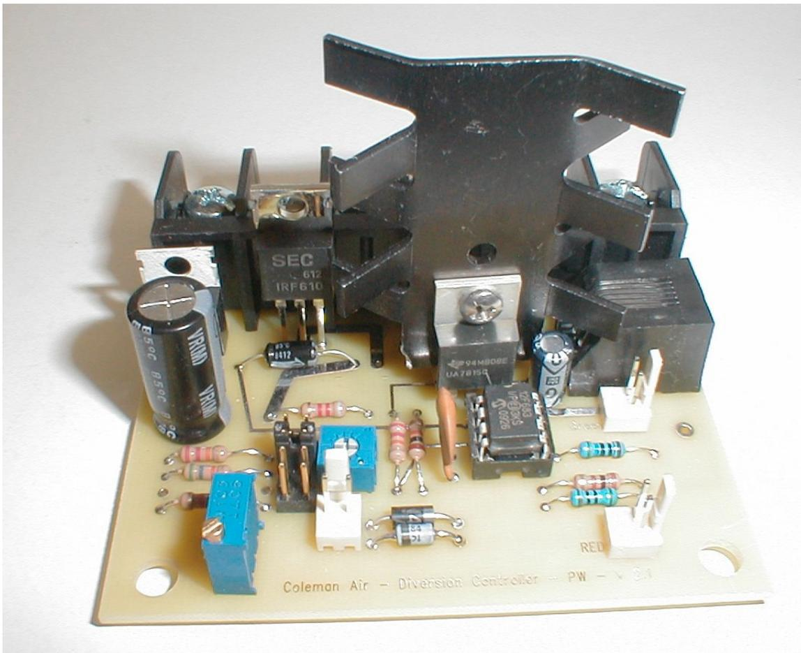
Completed board with heat sink properly installed on the regulator. Please note, some components may be in a slightly different position on your PCB. This can vary slightly from version to version.
